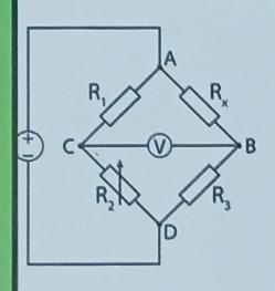
$$\frac{R_x}{R_1} = \frac{R_3}{R_2}$$
